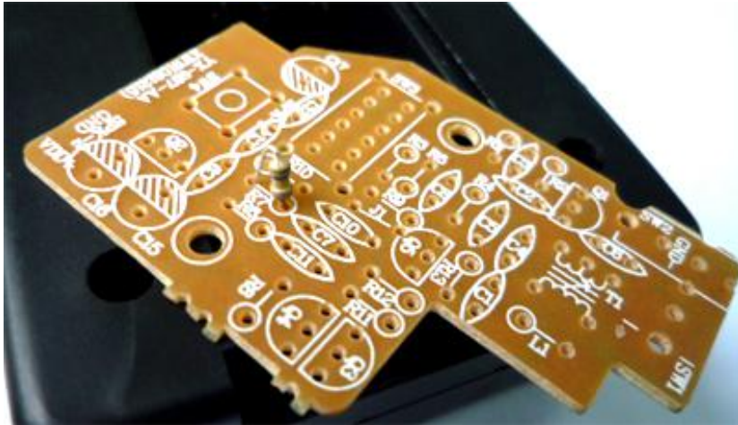
Vertical plug-in mounting of resistors
