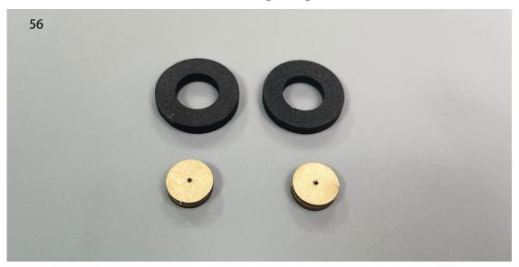
57. Assemble the hub and tire, securing with glue.
