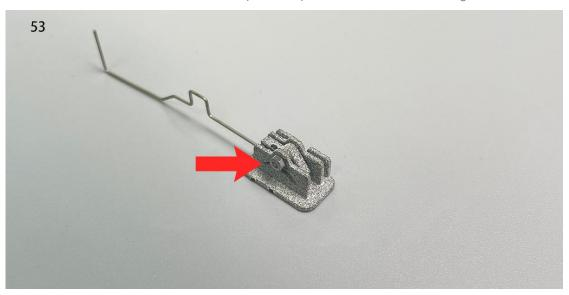
54. The landing gear on both sides is designed with mirror symmetry. Please assemble both sides of the landing gear in a mirrored symmetrical manner to avoid any confusion.
