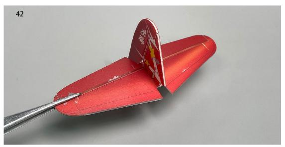
43. Attach the horizontal stabilizer to the corresponding location on the fuselage, ensuring that the horizontal stabilizer is parallel to the wing spar.
