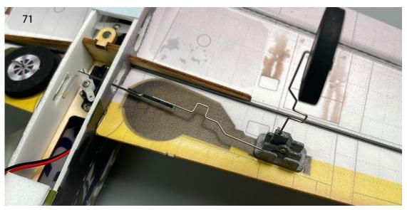
72. Install the other rod on the opposite side in the same manner, making sure the opening of the rod end clamp faces downward.
