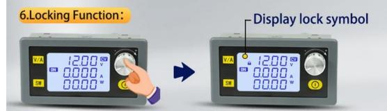
In the operation interface, long press the encoder button for 2 seconds to lock the voltage and current set to prevent misoperation; After locking, long press the encoder button for 2 seconds to unlock.
