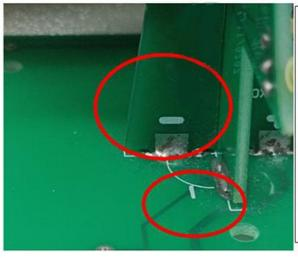
The negative electrode of plate B is installed on the negative electrode of the bottom plate and fixed by welding
