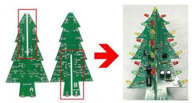
Step 2: There are solder pads where the A/B board is inserted. Please apply tin to fix the two boards.
