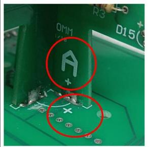
The positive electrode of plate A is installed on the positive electrode of the bottom plate and fixed by welding
