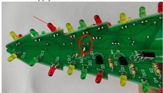
Step 3: After A/B are stuck together, take out the remaining lamp beads and select the color you like and solder them to the red position on the top of board A (pay attention to the positive and negative poles)
