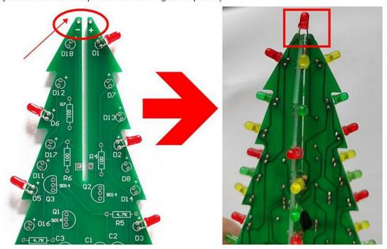
Step 4: After A/B are stuck together, solder them to the base board (Pay attention to the positive and negative poles)
