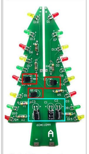
The electrolytic capacitor must reserve 1CM feet and lay it down at 90° close to the board after soldering.
