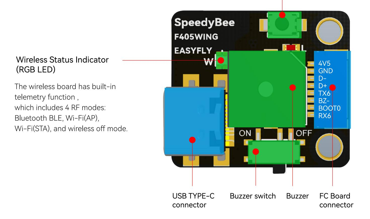
Green Slow Flash: Bluetooth BLE not connected Solid Green: Bluetooth BLE connected
