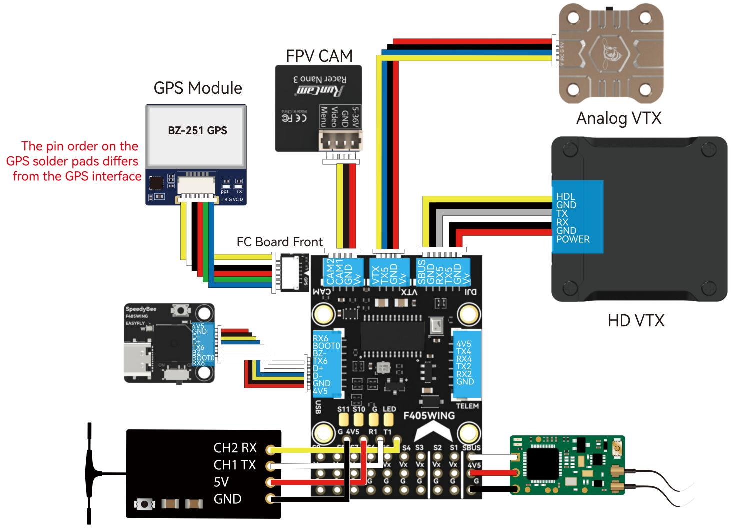
ELRS/TBS receiver Use a 4-pin Dupont female header on the FC Board front. SBUS/PPM receiver Use a 3-pin Dupont female header on the FC Board front.
