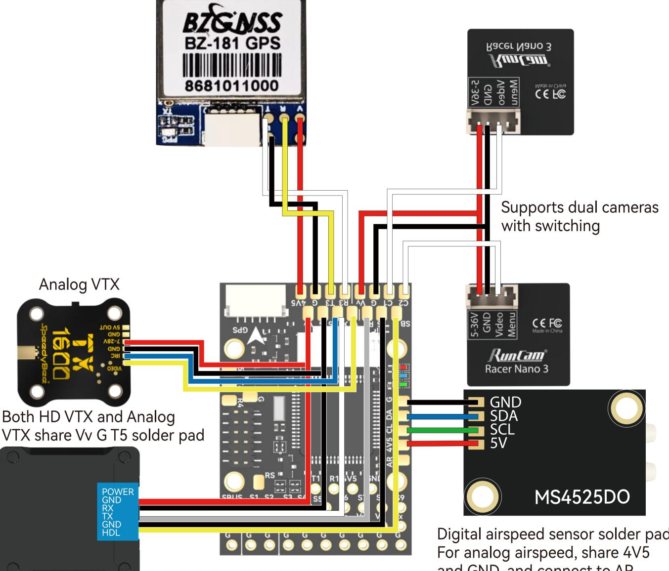
Digital airspeed sensor solder pad and GND, and connect to AR solder pad
