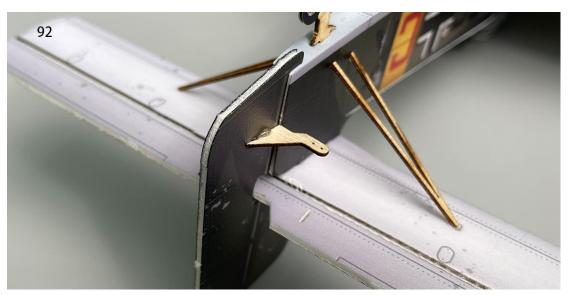
93. Install the elevator control horn.
