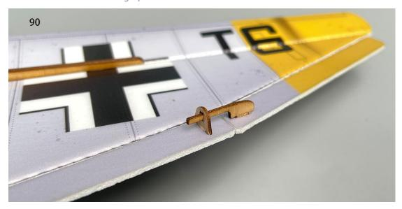
91. Install the aileron control horn.
