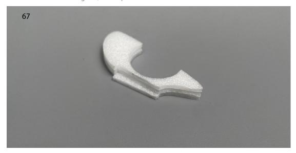
68. Assemble the PS foam board and printed KT board according to the corresponding outlines.
