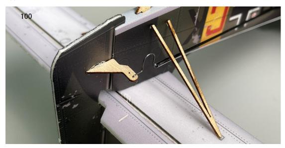
101. Cut a 40mm length of carbon rod for use as the aileron linkage. Use heat shrink tubing to connect the linkage to the servo wire clamp, and apply 502 glue to secure it.
