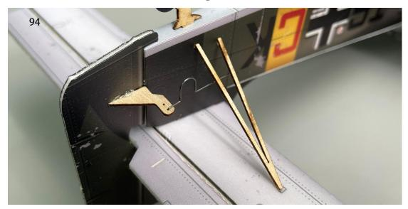
95. Install the elevator control horn connecting hook.
