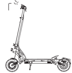
3.Tighten the screws and check the power switch.
