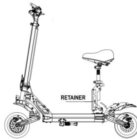
3. After pressing the lock pedal to bottom, slowly lower down the seat.
