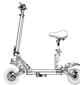
2. After standing up the seat bracket fully,Loosen the seat axis,fits that into slot.
