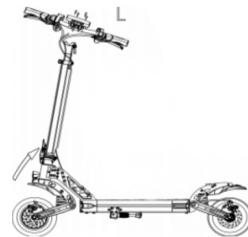
3. Flip the instrument forward, revealing the instrument screw hole and put the screws in it.tighten it by wrench, and then flip instrument backward,tighten screws by wrench.
