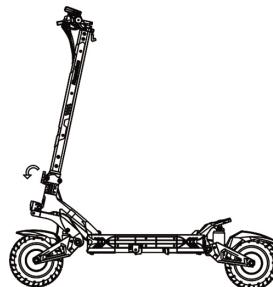
2. Hold the pole with one hand and pull the spring pin outward with the other.
