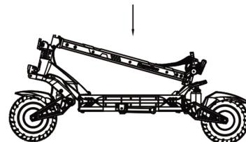
4. Adjust the body bars to make sure the hooks fit into the slots and snap into place.
