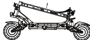
3. Straighten the body bar and apply force forward
