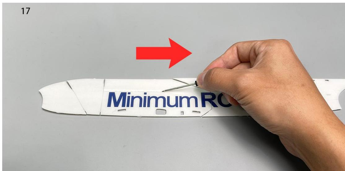
18. Caution: When performing scoring operations, make sure to press on the part closest to the lines to avoid tearing the components. (As shown in the diagram.)
