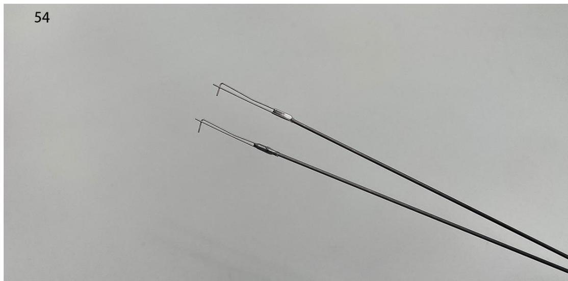
55. Cut out the top operation window cover to facilitate the installation of the horizontal tail fin control rod. Install the rod clamp head onto the tail servo arm.
