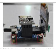
10. 用铜柱和 M2 4mm 螺母固定 PCB 四个角。 Fix the four corners of the PCB with copper posts and M2 4mm nuts.
