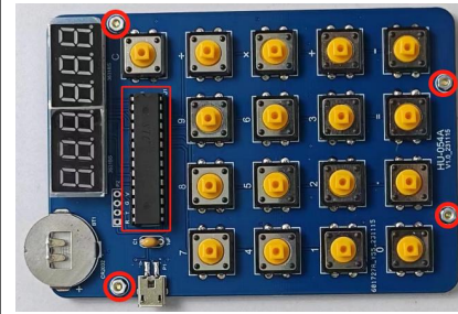
7. 把 STC15W408AS 芯片插到 IC 座上,并用铜柱和螺母固定 PCB。 Insert the STC15W408AS chip into the IC socket and secure the PCB with a copper pillar and nut .
