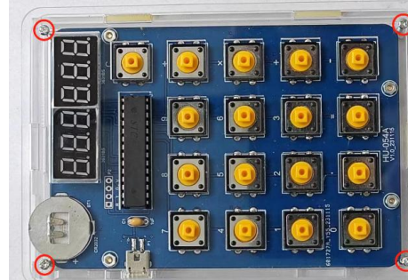
10. 组装好外壳,用 M2*18 的螺丝和螺母进行固定。 Assemble the housing and secure it with M2 * 18 screws and nuts.
