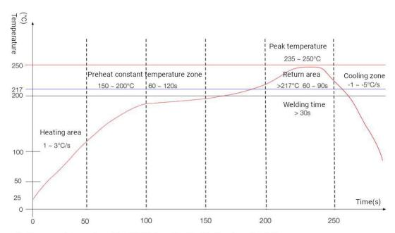
Heating zone -- Temperature:  $25 \sim 150^{\circ}$ C Time:  $60 \sim 90$ s Heating slope:  $1 \sim 3^{\circ}$ C/s
