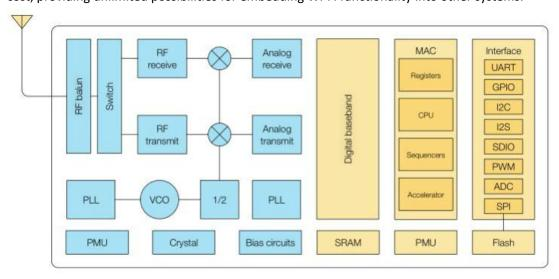
ESP8266 has a complete and self-contained Wi-Fi network function, which can be used independently or as a slave to run on other host MCUs. When used independently, ESP8266 can be booted directly from external flash. The built-in cache memory helps improve system performance and optimizes the storage system.
