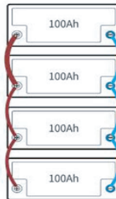
Parallel Connection 12V(12.8V) 400Ah
