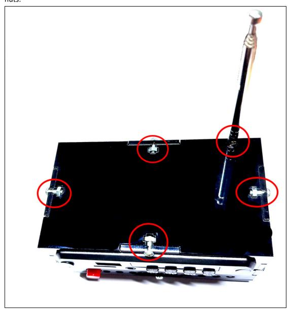
At this point, the outer shell is fully installed and can be plugged into a 5V DC power supply for testing.
