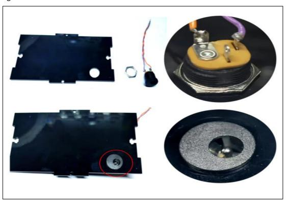
12. Weld the wires on the power socket to the position of the circuit board power solder joint
