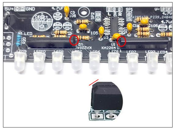
12. Install 5 4.7uF electrolytic capacitors. Note: The longer pin is the positive pole and connected to the "+" solder pad. The white side on the PCB board is the negative electrode.
