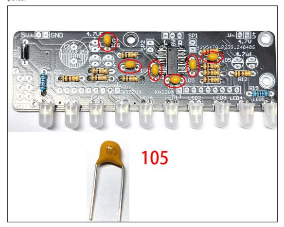
11. Confirm and identify the installation direction of KA2284, and install two KA2284 LED drivers on U1 and U2.
