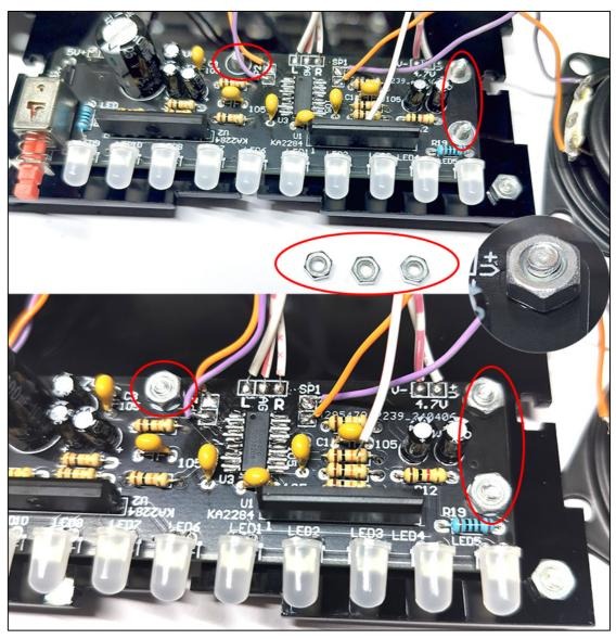
8. Install the multifunctional radio module onto the front housing using two M3  $\,^*$  8 screws and two M3 nuts.
