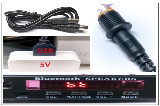
23. After powering on, you will hear sound and initially enter Bluetooth audio mode. Press the MODE key to switch.
