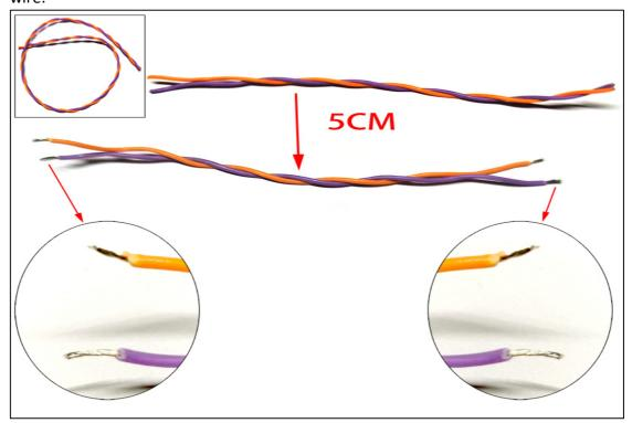
18. Connect the power button and PCB board with wires.
