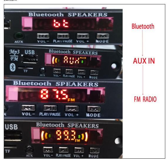
Bluetooth mode, which can be used as a Bluetooth speaker through a mobile phone Bluetooth connection.
