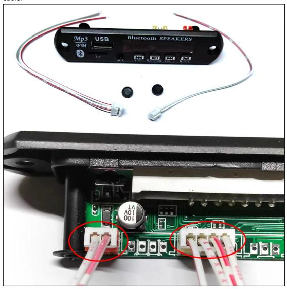
16. Weld the wires of the multifunctional radio module to the corresponding solder pads on the PCB circuit board.
