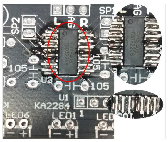
7. Weld low resistance components, 8 10K, 2 1K, and 2 100 ohm resistors
