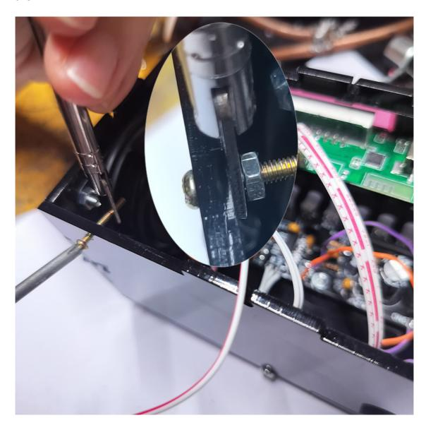
17. Use wire stripping pliers to peel off the insulation at the end of the wire connecting the antenna on the multi-functional radio module, exposing the copper wire. Then, wrap the copper wire around the M2 \* 16 screw and secure it with another M2 nut to prevent the wire from falling off.
