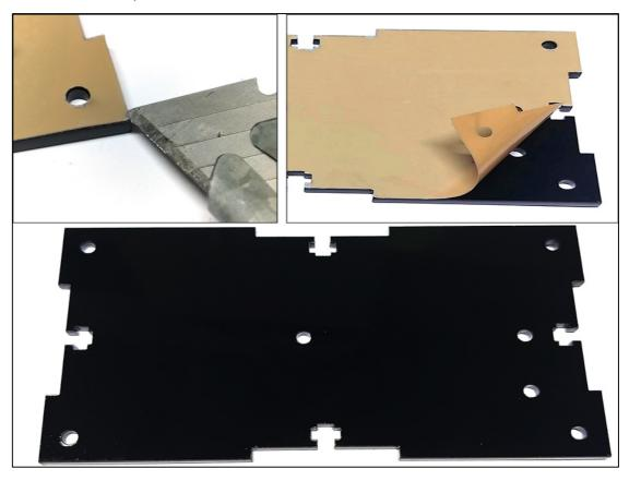
4. Find the bottom shell plate, tear off the film, and install 4 M3 \* 10 screws, 4 nuts, and 4 black foot pads.
