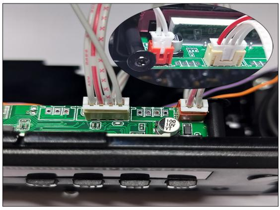
11. Install the DC022 power socket onto the back shell board, paying attention to the installation position of the power socket, as shown in the figure.
