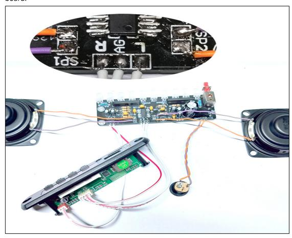
22. Now that all components have been connected, connect the 5V USB cable to test whether the module is working.
