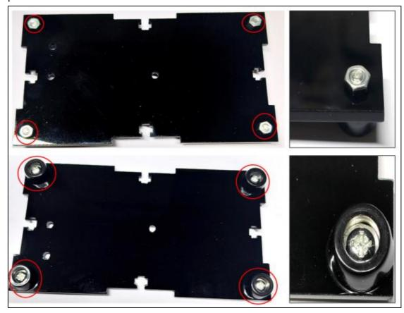
6.After installing the foot pads, find 3 M3  $^{\ast}$  10 screws and M3 nuts and install them on the bottom shell.
