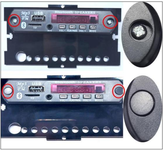
9. Use an M3  $^{\ast}$  8 screw and an M3 nut to install the front and bottom shells together.
