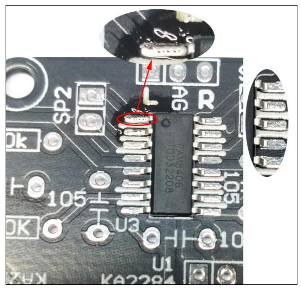
6. Use solder and soldering iron to connect the remaining pins of PAM8406 to the solder pads on the PCB.
