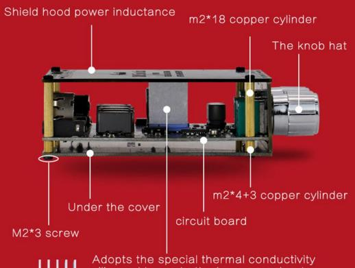
Adopts the special thermal conductivity silica gel to paste the large area heat radiator close to the shell of the copper heat dissipation area doubled to ensure that the product full power and high performance operation
