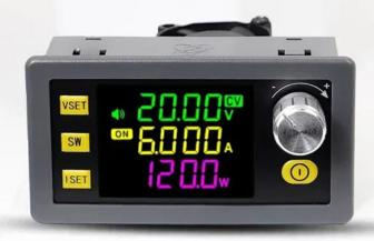
Fully protected: ☑ Anti-reverse ☑ Wanti-backflow ☑ Vunder-voltage ✓over-voltage ✓over-current ✓over-temp ✓over-power ✓over temperatur
