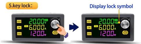
On the main UI, press and hold the encoder button for 2 seconds to lock the set voltage and current to prevent misoperation; press and hold the encoder button for 2 seconds after locking to unlock.
