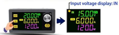
On the main UI, press the wbutton briefly to switch between input and output voltage displays.
