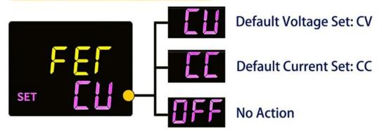
In the system parameter settings UI, set the parameter FET to CV or CC. Rotate the encoder on the main UI to enter the voltage or current setting UI. Rotate the encoder to quickly set the voltage or current.
