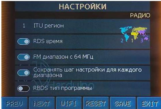
To enter setup mode, press the SETUP button on the main screen. Settings are divided into pages. Switching pages is done by rotating the encoder or using the PREV and NEXT buttons. Click WIFI for connection settings (page 15). Press RESET to load default settings. To save settings, press SAVE or EXIT and confirm saving.
