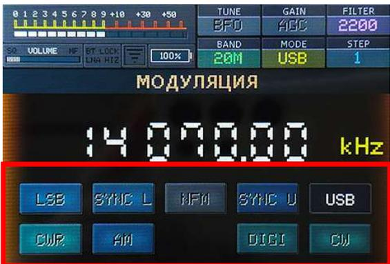
Types of modulation / decoder of Morse code and digital modes of communication
