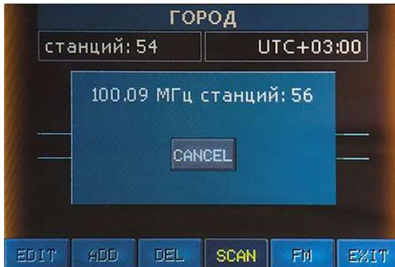
During the search process, the current frequency will be displayed and number of stations found. You can abort the search at any time without saving list of found stations by pressing the CANCEL button. When the search is complete, save the stations found. Then press the FM button and change the station names created automatically. You can edit list on your computer (page 19).
