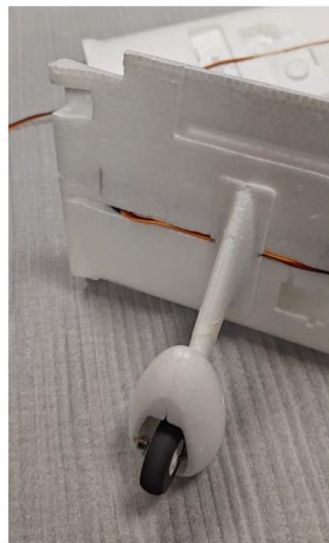
Fix the steering gear, steering gear line and landing gear with foam
