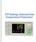
Press the power button briefly to enable/disable the external over -temperature protection function, which is defaulted to "off" when disabled.
