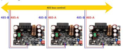
Independent dual serial ports (usable simultaneously) featuring serial TTL level communication and onboard 485 communication.
