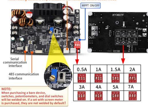
ON: NC Mode, controlled by meter or Modbus OFF: Potentiometer Mode, adjust voltage by rotating the potentiometer, and set the constant current value through DIP switch.
