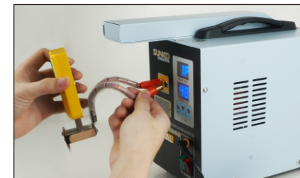
2. Copper wire plug in the welding head
