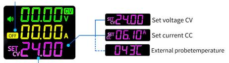
When the power is off, the set voltage and currentare displayed downward in turn.
