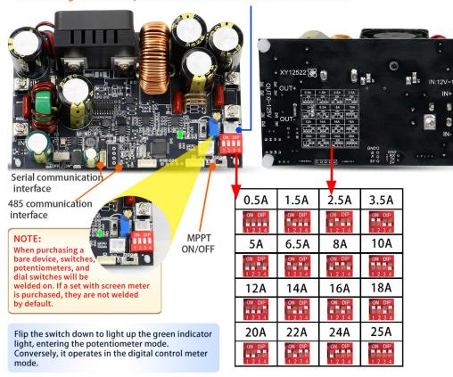
In potentiometer mode, the output voltage (constant voltage) can only be controlled through the potentiometer; the constant current value can be set via a dip switch, with a total of 16 gears to meet most scenarios (can also be set via Modbus).
