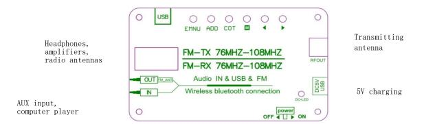
Power on: Turn the switch POWER to the left OFF position to turn off the power, and the right ON position to turn on the power.
