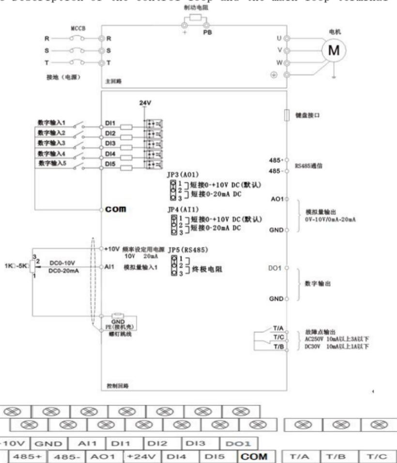
Figure 1-3-1 0.75-11.OKW wiring diagram control terminal description
