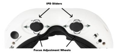
The suggested method for optical adjustments is to first power on the headset and get a stable image. This can be done by using a VRx with an external camera, the AV in, or even the DVR menu. Once you have a stable image go through the following steps:
