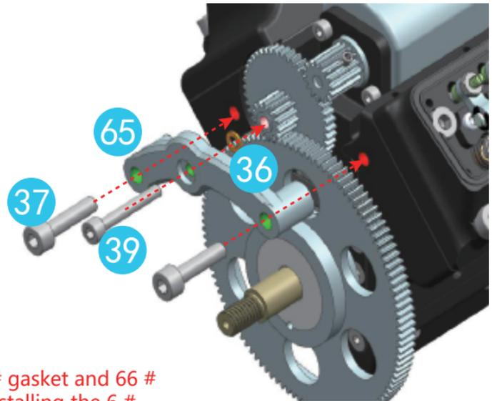
\*The 39 # screw passes through the 65 # part, 36 # gasket, 66 # gear, and 36 # gasket in sequence. Two 37 # screws pass through the 65 # part and are finally fixed on the cylinder block
