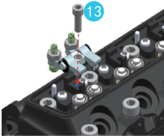
\*Fix the rocker arm bracket assembly with 13 # screws and adjust the valve clearance with 16 # nuts, ensuring that there is at least 0.1mm clearance between each rocker arm and valve
