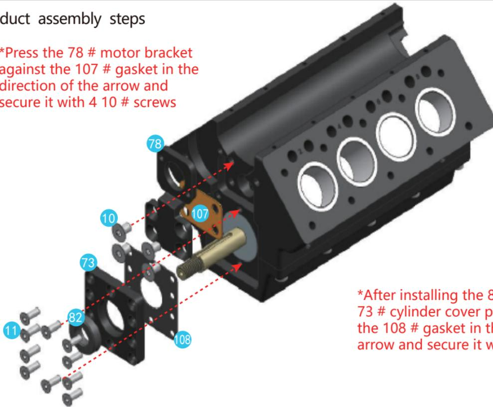
\*After installing the 82 # oil seal into the 73 # cylinder cover plate, press down on the 108 # gasket in the direction of the arrow and secure it with 10 11 # screws
