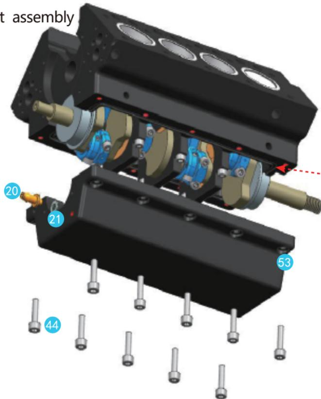
Seal the groove position with glue
