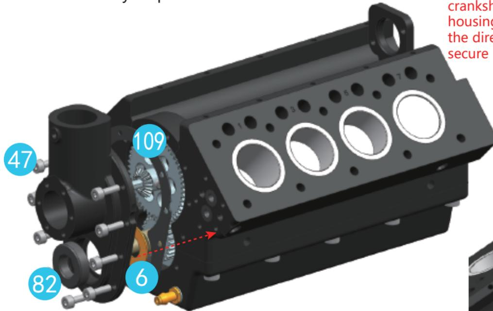
\*Insert the 82 # gasket onto the crankshaft, press the 47 # distributor housing against the 109 # gasket in the direction of the arrow, and secure it with 9 47 # screws
