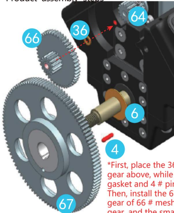
\*First, place the 36 # gasket and 66 # gear above, while installing the 6 # gasket and 4 # pin on the crankshaft. Then, install the 67 # gear. The outer gear of 66 # meshes with the 64 # gear, and the smaller inner gear meshes with the 67 # gear
