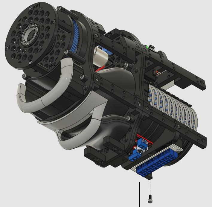
Attach both DC Motor wires to the L298N DC Motor Driver on terminals "Motor A".
