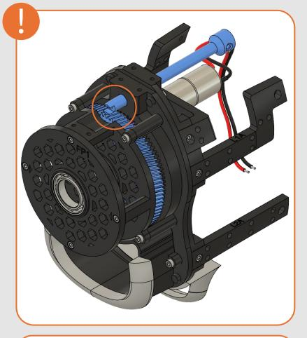
Loosely insert "PROP CONTROL SHAFT" as shown. We will attach it in the next section.
