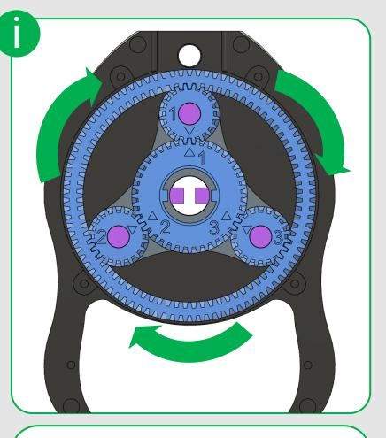
Rotate "PROP CONTROL RING GEAR" to ensure smooth movement. If not, you may be off by one tooth. Remove and resit. Return both sun gears to original position as shown:
