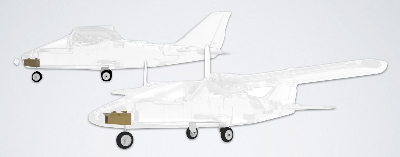
Modular landing gear: Front and rear landing gear set.
