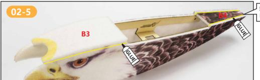
粘贴B3,B4在机身顶部。 Paste B3, B4 at the top of the fuselage.
