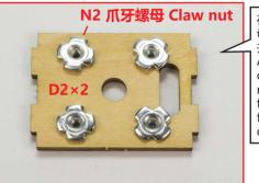
在机身头部粘贴马达防火板,注意装有螺母一面朝机身内。防火板2片粘在一起,并装爪牙螺母。 Attach the motor firewall to the head of the fuselage, pay attention to the nut side facing the inner of the fuselage. The two pieces of the firewall are glued together and the claw nut is installed.
