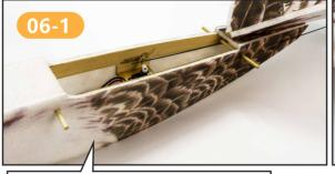
把机翼放置到机身居中位置,用橡皮筋锁定机翼。 (如上图所示) Place the wing in the center of the fuselage and lock the wing with rubber band as shown above.
