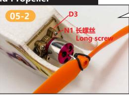
把马达固定到防火板上。此时根据你所选马达的大小垫入D3,调整到合适长度。 Secure the motor to the firewall. At this time, according to the size of the motor you selected, pad D3 and adjust to the appropriate length.
