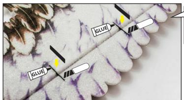
在副翼处切小口,嵌入碳片, 用胶水粘固,即可封闭副翼。 Cut a small opening in the aileron, insert a carbon sheet, and glue it to seal the aileron.
