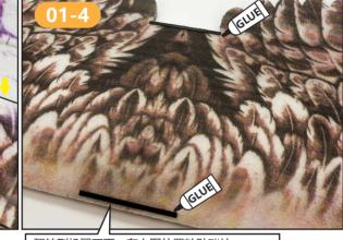
把粘合好的机翼反转到反面,在预留槽内嵌入碳片,用胶水粘牢固。 Reverse the bonded wing to the reverse side, insert the carbon sheets in the reserved groove, and glue it firmly with glue.
