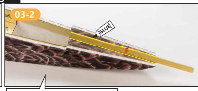
在机身尾部粘贴三角木(如上图所示)。 Paste the triangle wood at the end of the fuselage (as shown above).
