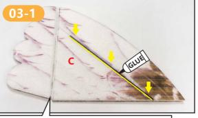
在尾翼预留槽内嵌入碳片, 用胶水粘固。 Insert a carbon sheet in the reserved groove of the tail and glue it with glue.
