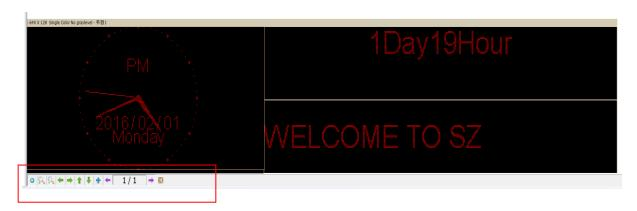
Notice: see the red place, there have tools for edit simulating screen. (Include tools: preview/pause preview, zoom in/ zoom out simulation window, current region right and left shift, region overall, display content paging, simulate display window top left corner display )
