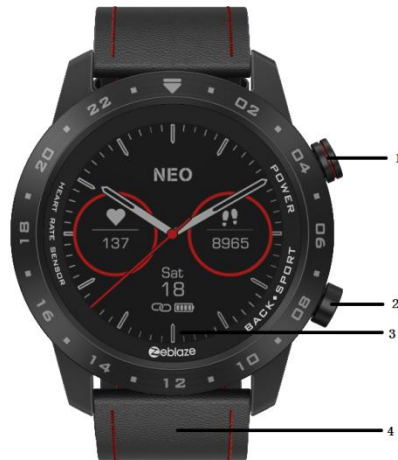
1 Power on/off key 2 Side-down key 3 Display 4 Watch strap
