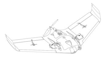
The specially air-cooled side bays open to the sides for you to place any gear you want.
