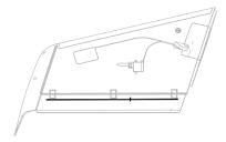
Glue the carbon fiber spar and control horn for aileron enhancement.
