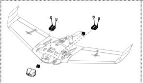
This unit is especially designed to host the DJI HD FPV system. You have a top hatch and a nose dedicated for it. You can also place the DJI system on the side bays, but we recommend you to use the central placement for better cooling and horizontal balance.
