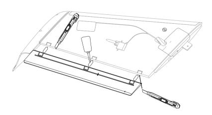
If you plan to install the provided CA hinges, please cut the EPP following the markings on wings and elevons for a proper alignment. Also make sure you leave around 1mm clearance between the elevon and the trailing edge of the wing so the control surface can move freely. Don't overdo with the glue!
