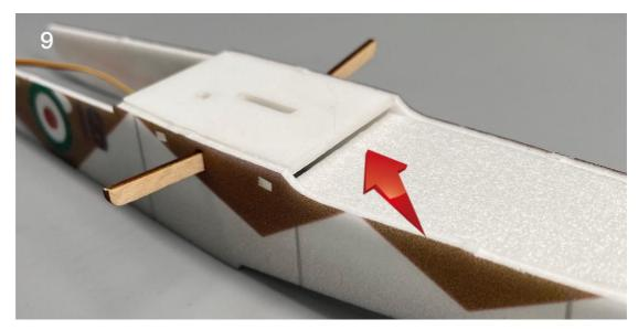
10. To install the bottom plate of the hull head, the plate can be bent in advance before installation.
