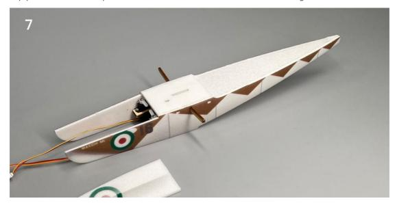
8. Details: the top plate in the middle of the hull shall not interfere with the movement of the steering arm.
