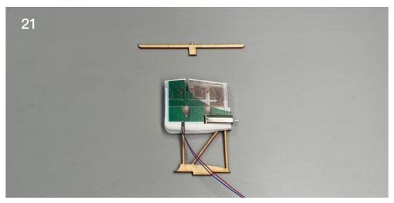
22. Install the spar. Please keep the spar perpendicular to the motor base.
