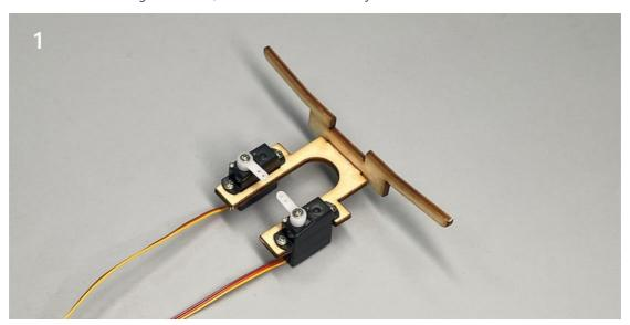
2. Combined servo seat and hull side plate.
