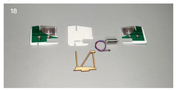
19. Align the bottom and glue the middle and right motor base parts. Note: there is a height difference of 2mm at the top of the two panels.
