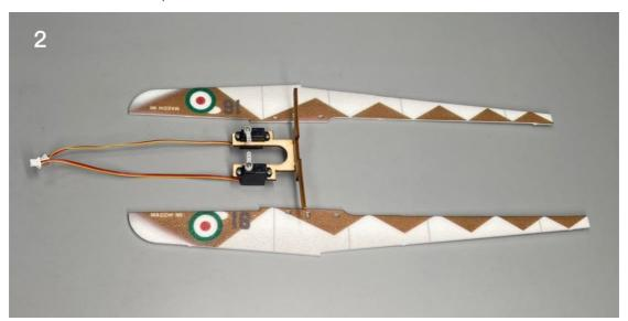
3. Details: the bottom of steering gear should be 2mm away from the edge of hull side plate.
