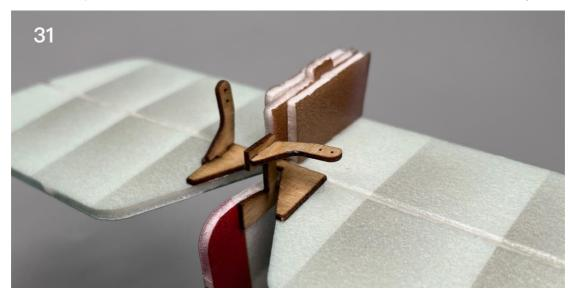
32. Install the tail assembly and paste the tail side sticker. Make sure the horizontal tail is parallel to the fuselage and the vertical tail is vertical to the fuselage
