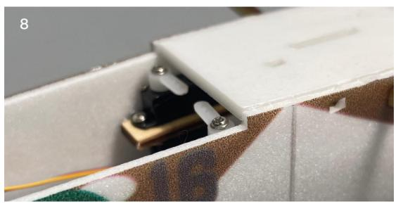
9. Details: there should be a gap between the middle part of the hull and the tail roof to allow the push rod to pass through.
