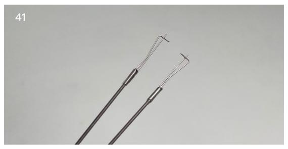
42. Extend the carbon rod of the pull rod from the slot at the middle and rear of the hull, and use tweezers to fasten the steel wire clamp on the hole of the servo arm.
