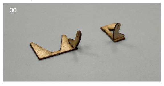
31. Glue the control horn parts on the tail. Please make sure that the elevator and rudder can move freely.
