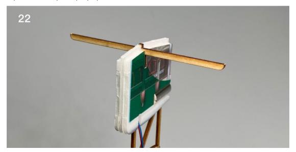
23.Use the end of a carbon fiber rod to score through the half-cut line of the wing surface.
