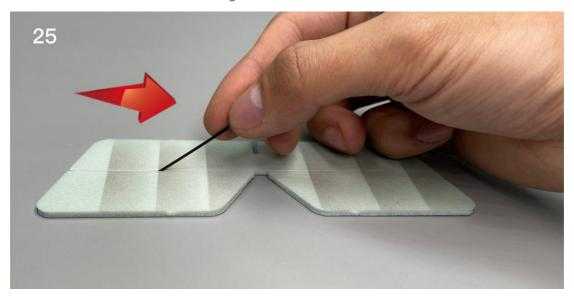
26. Use the end of a carbon fiber rod to score through the half-cut line of the rudder surface.
