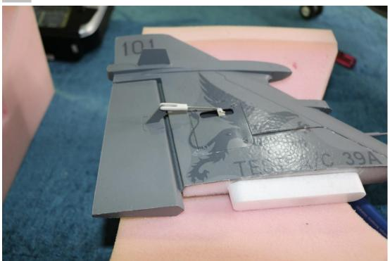
14: Connect the servo with the extension wire, and pay attention to the corresponding positive and negative poles. Secure the excess wire with tape or tie.
