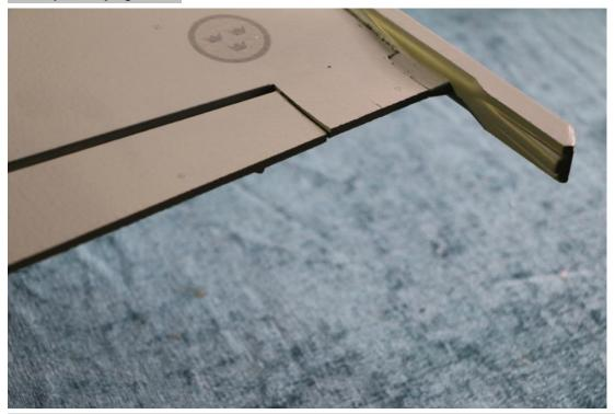
26: The canard can be kept flush with the platform. Or the front end can be appropriately down 1 degree. If the canard tip is cocked, it will facilitate the take-off, but it can cause the aircraft to head up when high-speed flight.
