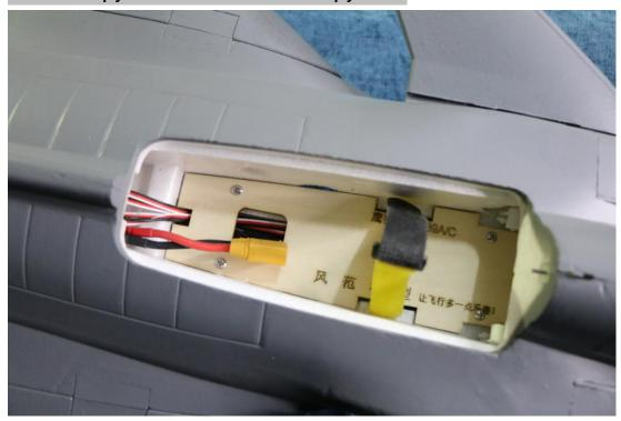
24: Fix the battery and charge to adjust the rudder surface. The battery compartments can hold up to 4700mAh 6S batteries.
