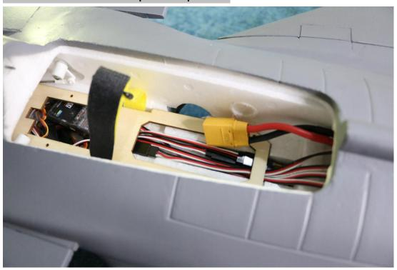
23: Install the plywood. All wires walk under the ply wood.
