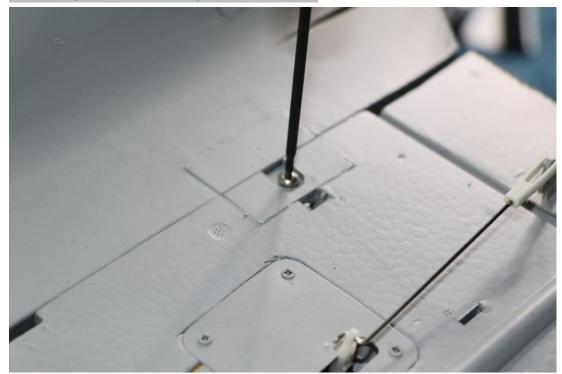
18: Glue the nose landing gear cover and ESC cover.
