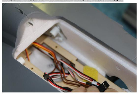
3: Power servo back to the neutral point and install the rod adjuster, The middle hole on the servo arm needs to be reamed with a 1.8mm drill. Then fix the servo with screws.
