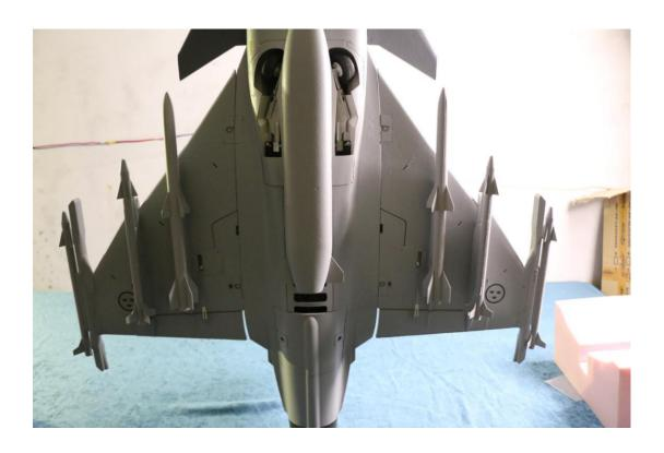
28: The center of gravity of the aircraft is at the joint at the end of the battery compartment cover.
