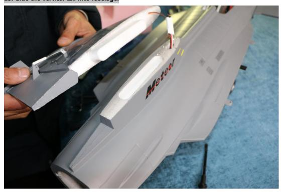
16: Adjust the length of the pull rod, install the pull rod and fasten the chuck. Plug the carbon rod into the wing and connect the extension cable, fix the extra cable with tape or tie and plug it into the reserved hole of the fuselage.
