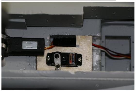
5: Power the two canard servos back to the neutral point and install into the servo holder with screws. (If the canard is used as the flap, follow up and down, then use 1 forward and 1 reverse servo. If the canard is operated with the elevon at the same time, then use two forward or two reverse servos).
