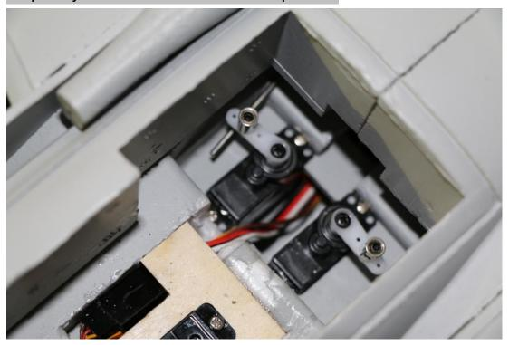
9: Adjust the length of the pull rod and hook the ball head on the canard rocker arm.
