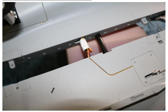
17: Fix wing with corresponding hex socket screws.
