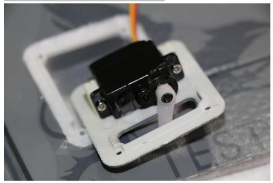
13: Power the two wing servos back to the neutral point. The outermost hole on the wing servo arm needs to be reamed with a 1.2mm drill. Adjust the length of the pull rod, install the pull rod, buckle the chuck, and fix the servo holder. (The two wing servos all use forward servo).
