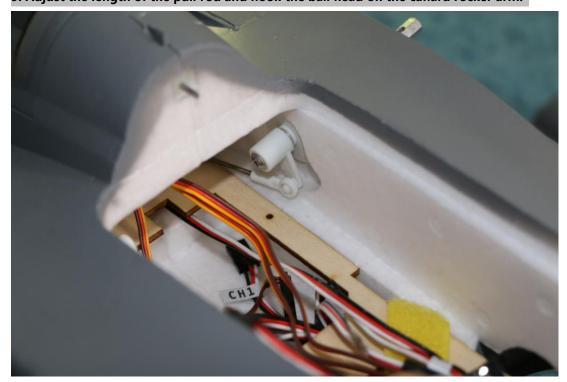
10: Adjust the length of the pull rod, tighten the inner hexagon screw to fix the canard pull rod.
