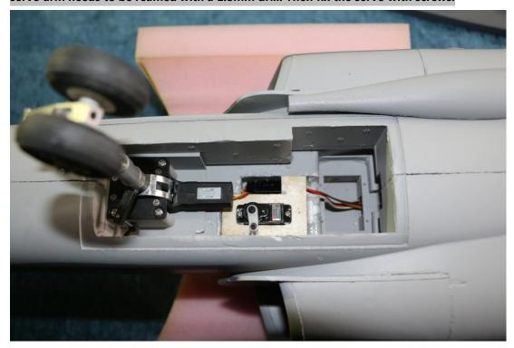
4.Adjust the servo and install the steering pull rod. Pay attention to the position of the servo arm. (The servo is forward servo.) The servo wire pass through the side open.
